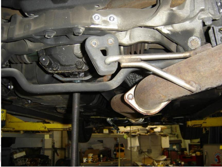
Remove the rear sway bar mounts from subframe & let hang, support the diff with a jack stand.
