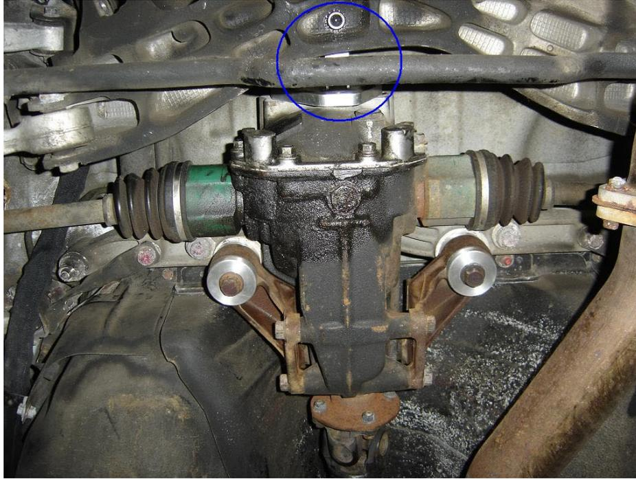
Mark the approx position of the threaded hole in the mount (front to back) onto the subframe (dark circle). Use pictures as reference only.
