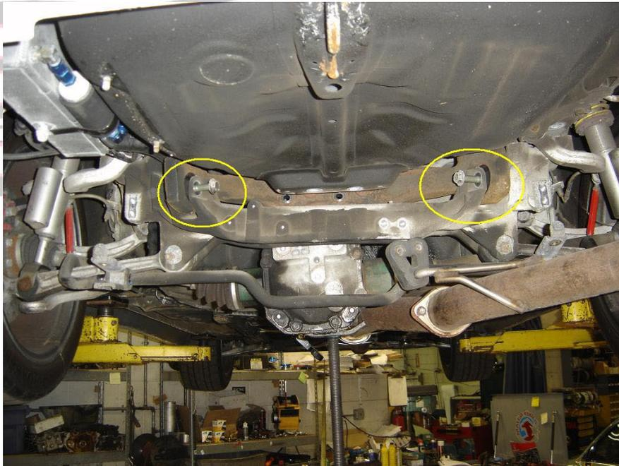
Loosen bolts at the ends of the mustache bar. (light circles)
