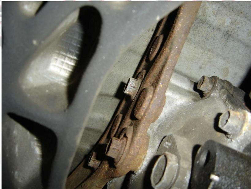
Remove the 3 bolts holding the mustache bar to the diff cover
