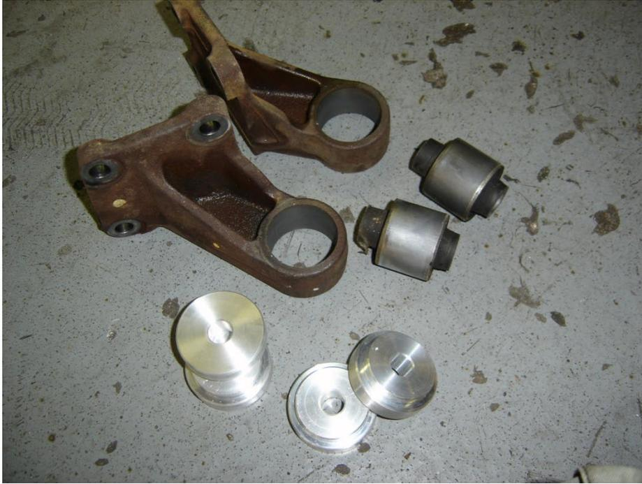
Using a press, remove the factory bushings from each diff mount ear.
