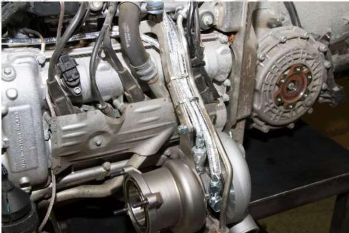
27) Next use the stainless steel ties to attach the lines to the support bracket. Make sure all the lines are as low as possible.
