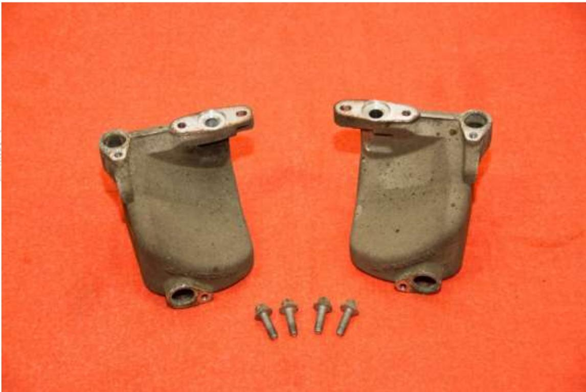
9) Once the turbos are removed, remove the oil drain tanks. These will be reused on the Alpha turbos using the original hardware. A new drain o-ring is supplied to replace the old one.
