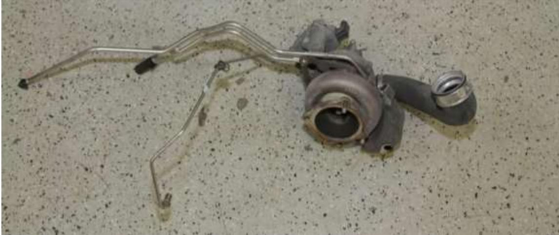
8) Remove each turbo with the coolant and oil feed lines.
