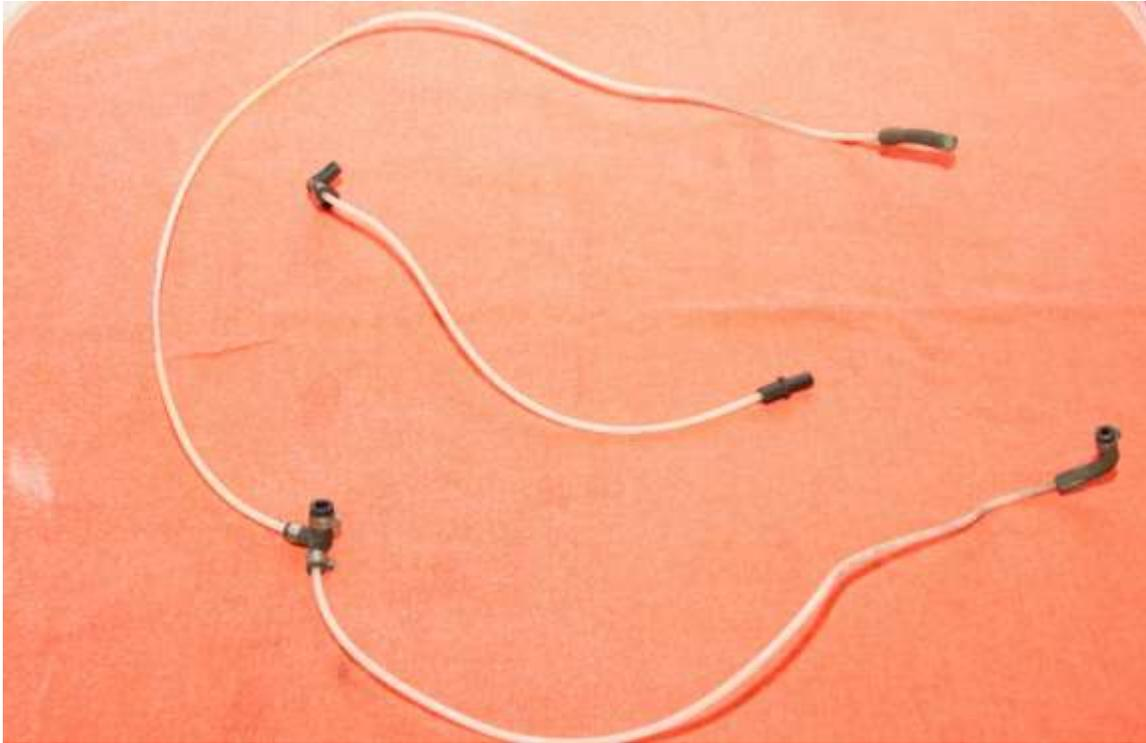
12) Remove the white plastic air tubes running from the factory turbo bypass valve to the control solenoid. The lines can be removed but the solenoid will remain in place and plugged in to avoid and check engine lights. Boost control must now be done by an external controller and will be covered latter in the install.
