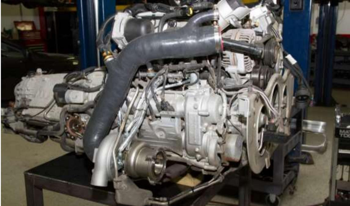
57) Next install the turbo inlet tubes. Install the turbo inlet tube with the gold quick connect fitting on the Driver's side and connect the factory breather hose. Install the other turbo inlet on the Passenger's side. Keep the turbo inlet tubes as close to the motor as possible.
