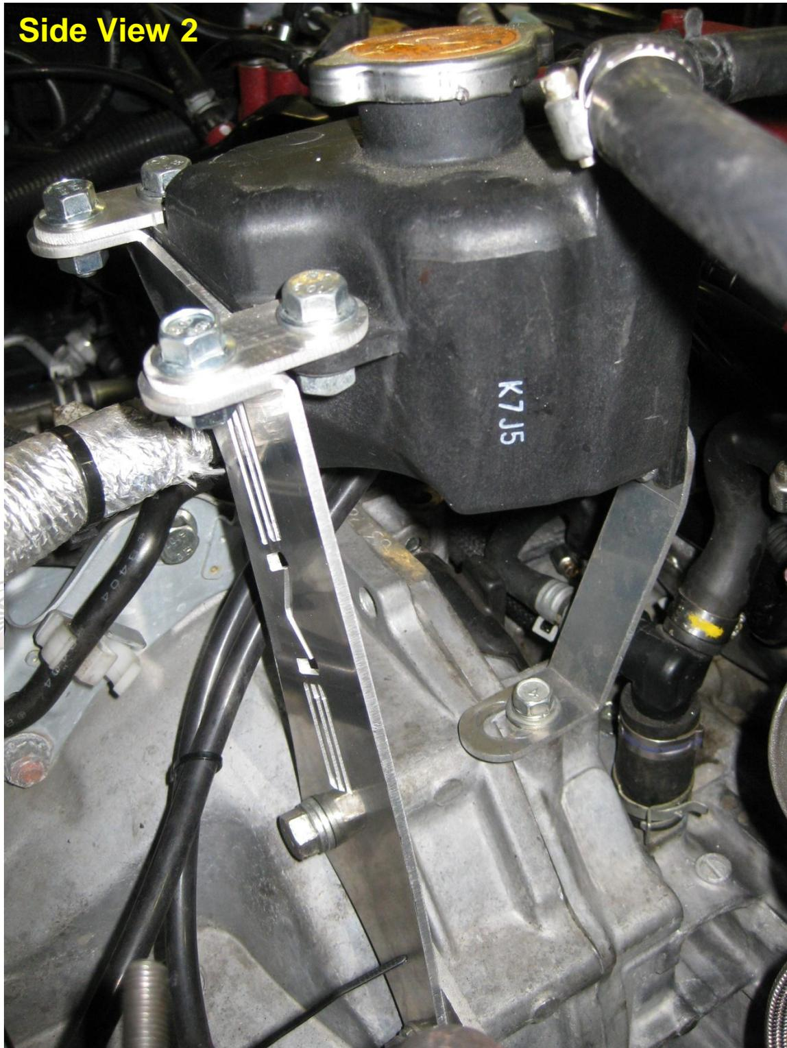
Install the brackets as shown with the large "AMS" one being stacked behind the turbo kit up-pipe support bracket on the transmission. Make sure to keep ALL lines away from any sources of high heat and/or abrasion using protective heat sleeve where necessary.
