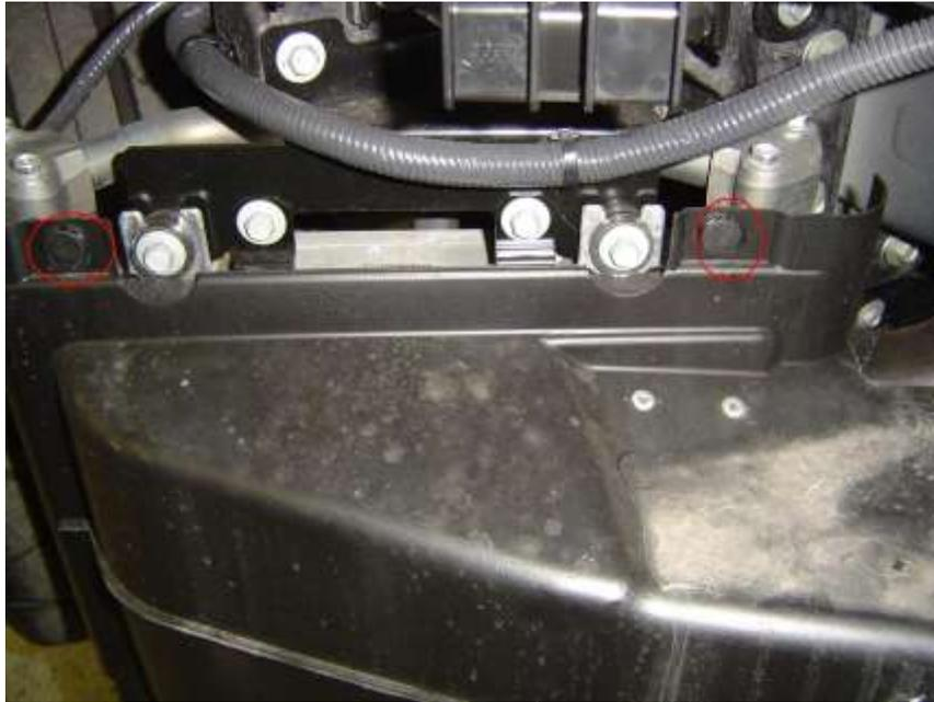
9) At this point you can remove the factory intercooler piping and install the AMS kit as shown below. We have found that when installed as shown the kit fits very well on most cars, in some rare cases fitment is found to be better by flipping the mid and lower pipes. Install the kit so it fits your particular car best. Some things to keep in mind during install are clearance around oil cooler and radiator shroud, and clearance from the wheel wells.
