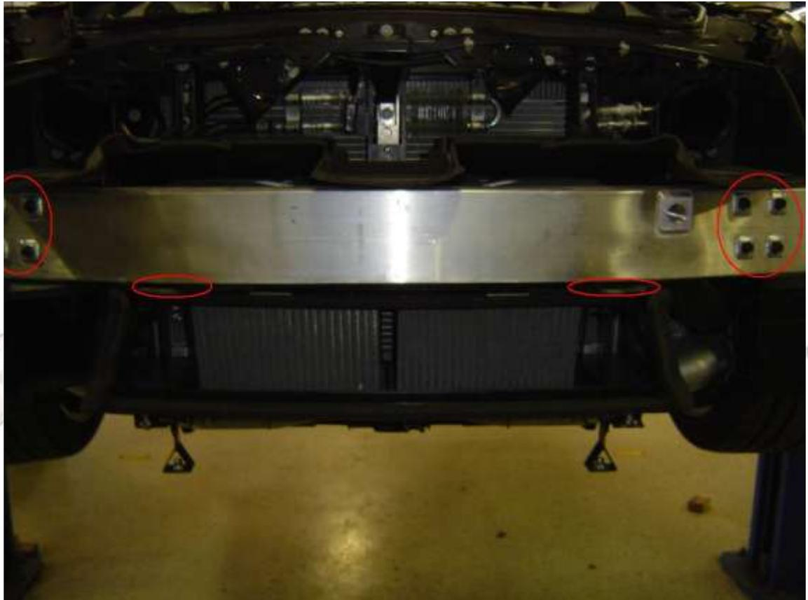
8) Remove oil cooler ducting by removing 4 clips.
