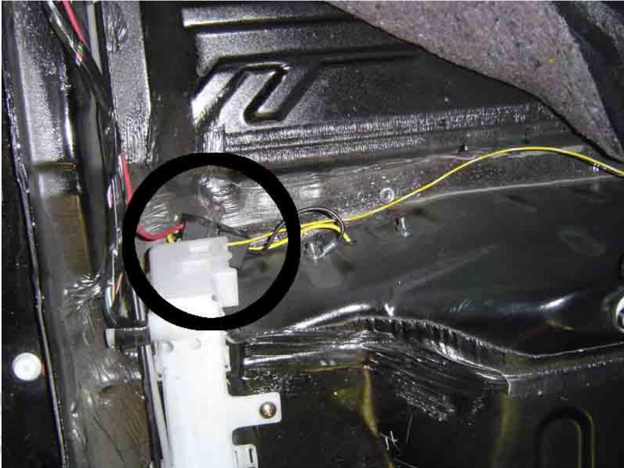
2. Drill (2) more 1/4" holes and install grommets supplied. Run thick yellow wire through hole towards pump and attach to positive on pump.
