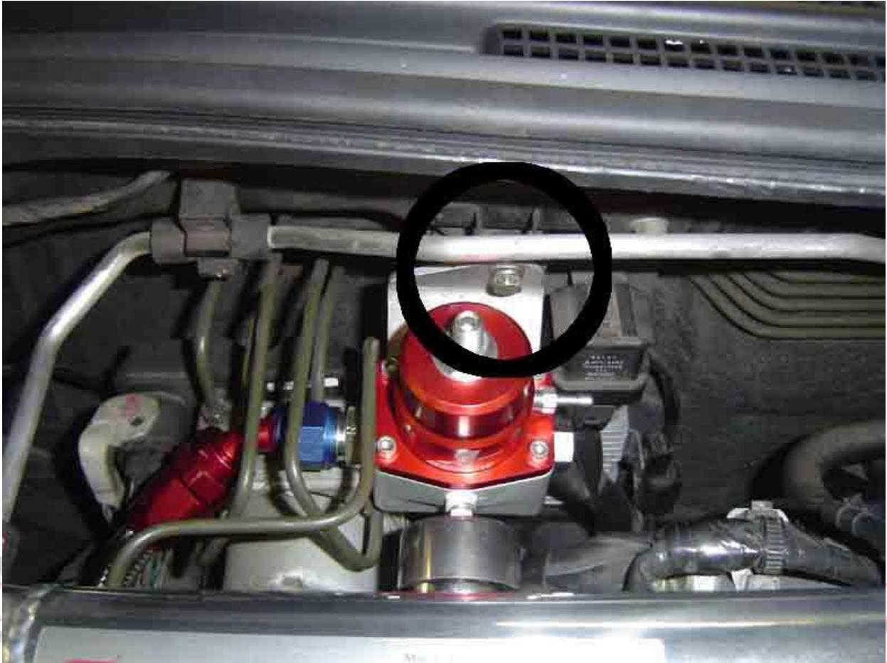
**\*\*Note\*\*** On ACD Cars you must move relay to gain access to bracket for Fuel Pressure Regulator .
