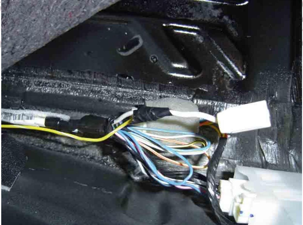
6. Remove door still plates and B pillar trim. Run red wire from relay along floor towards the front of car.
