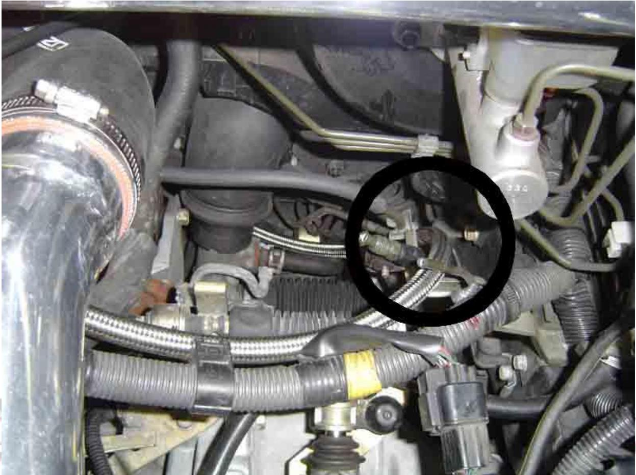
9. Remove return line from steel line under brake master cylinder. Cap off steel line with cap supplied.
