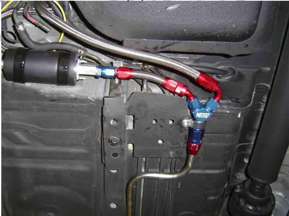
26. Remove plastic line under car that connects the two steel feed lines together. Install -6 braided line with quick connector on one end and 120 deg on the other end to steel line coming from sending unit to NOS Y. Cap off return line with supplied cap.
