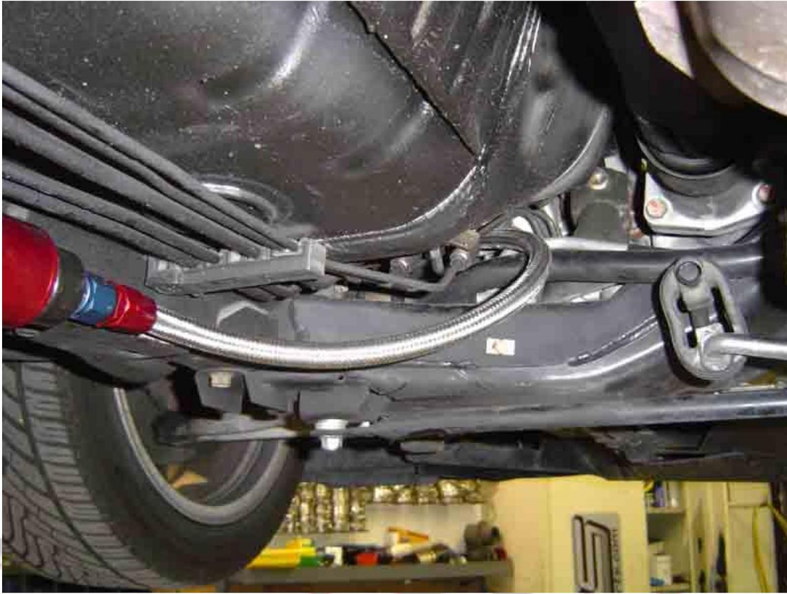
24. Install walboro external pump using supplied clamps. Find suitable location under car. Drill  $\frac{1}{4}$ " holes through floor and bolt the clamps to the underside of floor. Make sure pump is installed with electrical terminals facing passenger side.
