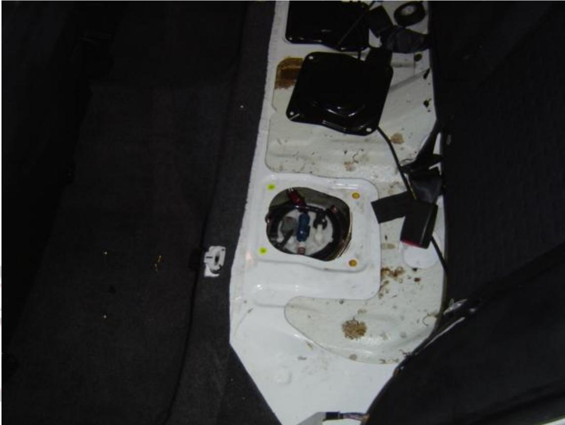
5. Disconnect lines and electrical connector to sending unit (Use rag around hoses to prevent fuel spray)
