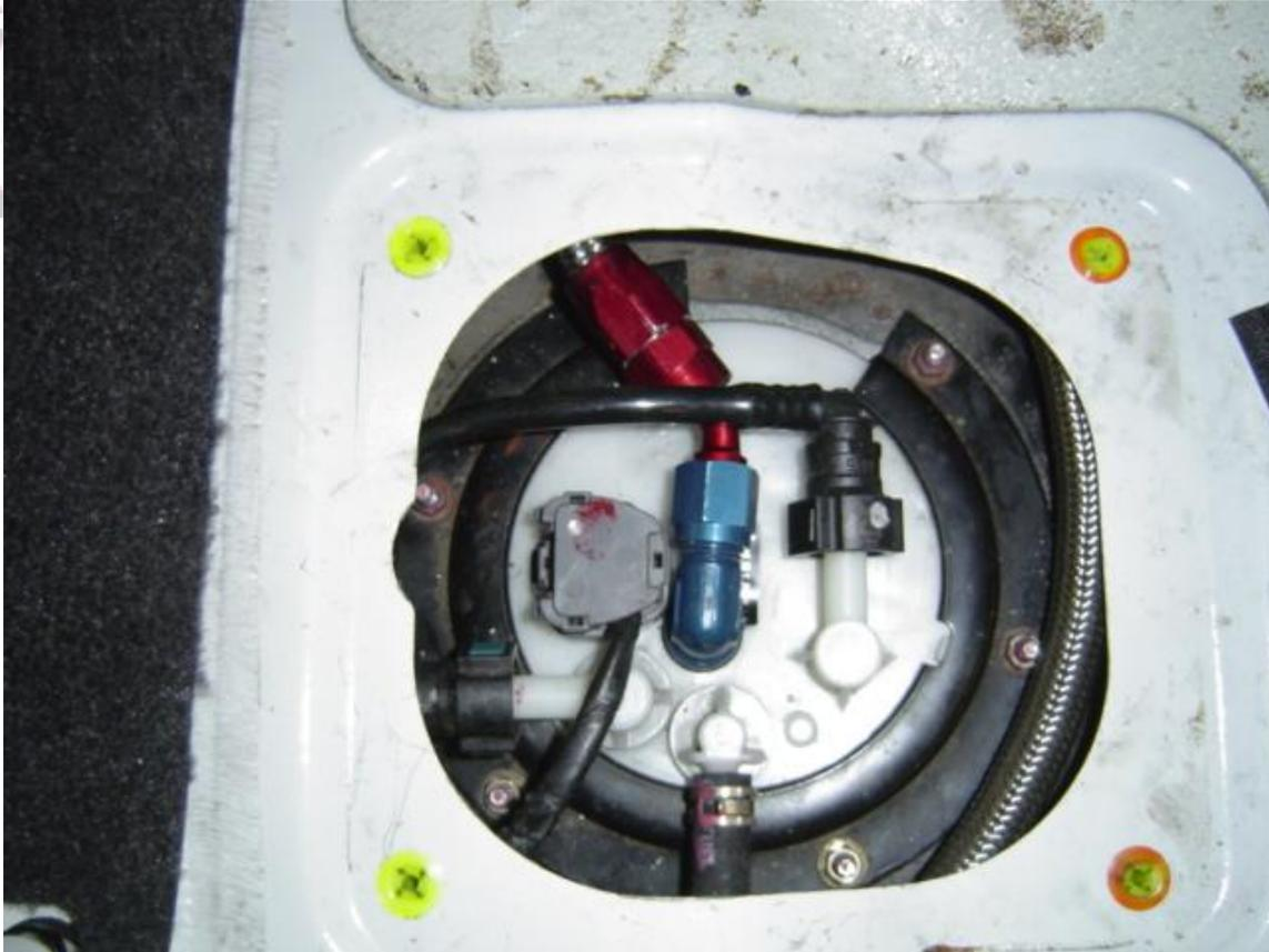
11. Reinstall gas cap and cycle key a few times to verify pumps are working. Check for leaks and start vehicle. Once vehicle is running, remove vacuum hose from fuel pressure regulator and set pressure to 43 PSI. Reinstall hose.
