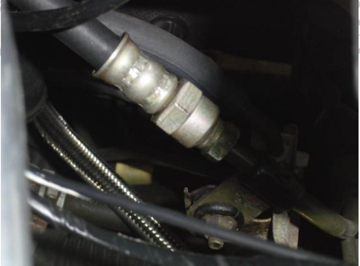
15. Find longest -8 hose with 45 deg on one end and to straight on other end. Connect 45 deg to the fuel rail inlet side near throttle body and run the rest of the line down firewall towards frame rail.
