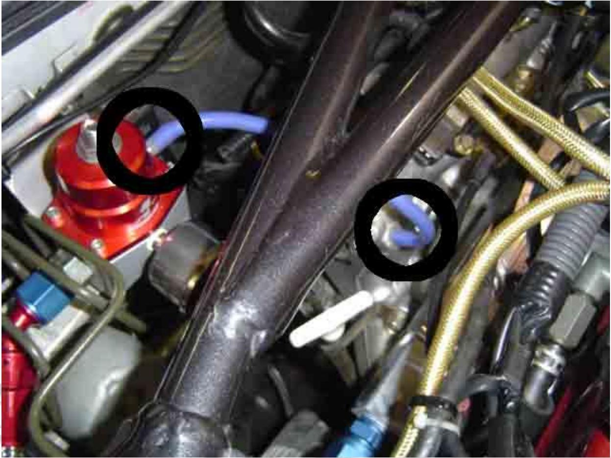
14. Use supplied 3/8" rubber hose and connect one end to the outlet on bottom of fuel pressure regulator with a clamp connect hose with the steel fitting on the end to stock feed line. Use barbed fitting to connect the 3/8" hose to the rubber end of the feed line using clamps.
