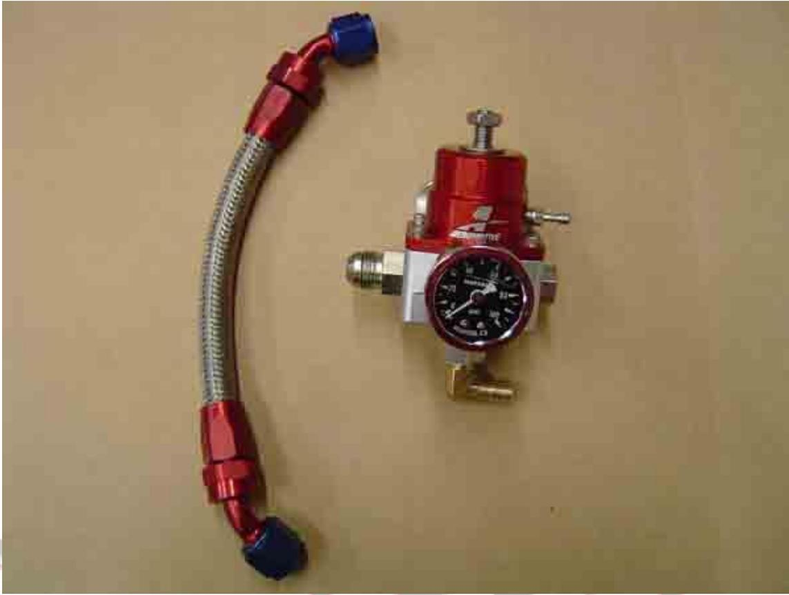
12. Install new fuel pressure regulator using supplied bracket on bolt by ABS as shown in picture
