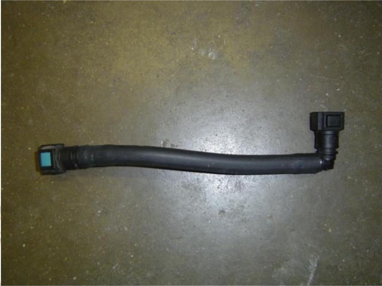
27. Use rubber 5/16" hose with 90 deg quick connect and connect feed line to return line going to sending unit.
