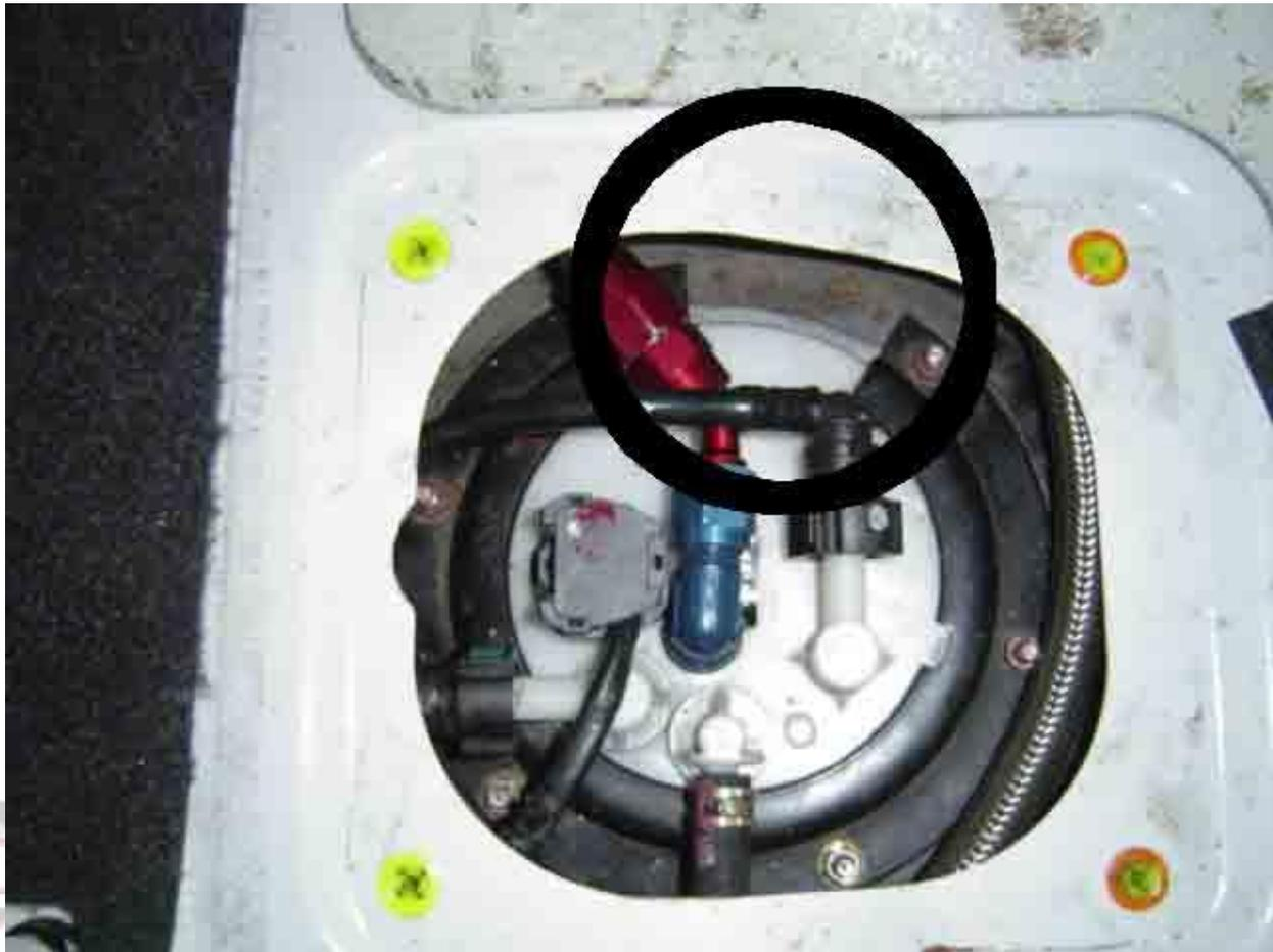
7. Carefully install supplied sending unit and plate with the cut section of plate facing passenger side tighten bolts leave lines off for now.
