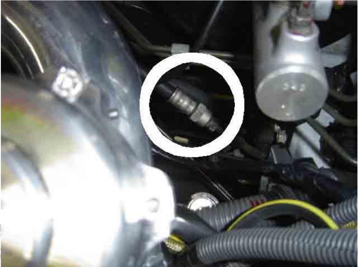
10. Remove stock feed line from steel line under master cylinder.
