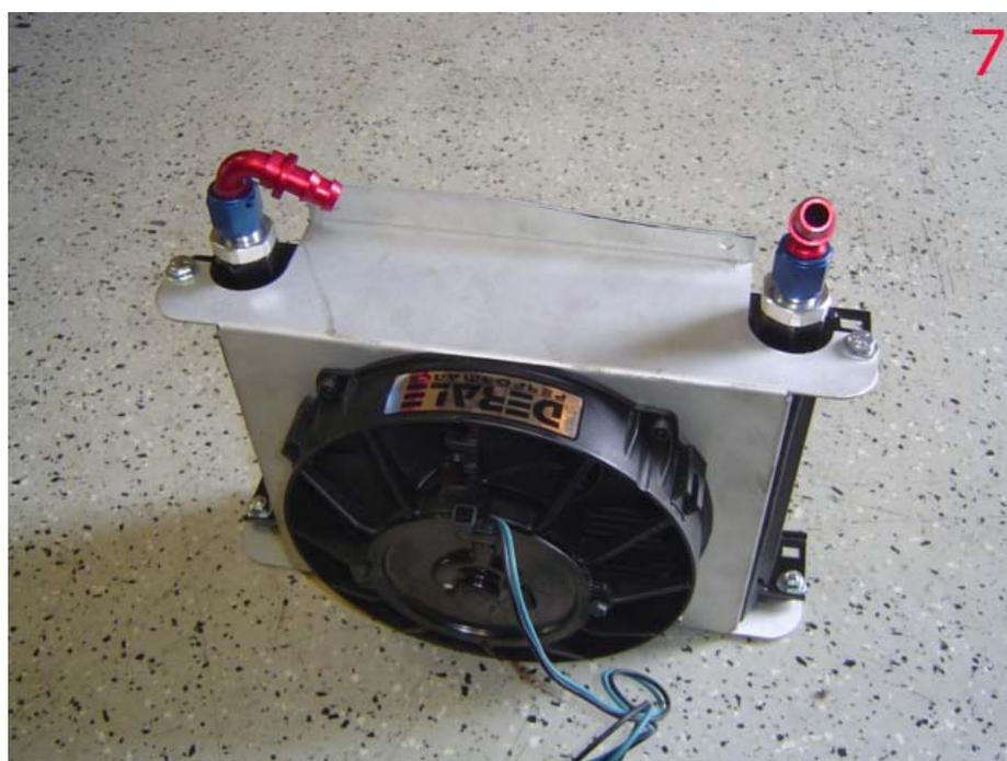
8. Now loosely install the cooler and cut the hoses so they can be pushed onto the fittings while still allowing enough movement to not put tension on the hose. The long hose goes to the top fitting. In most cases the longer hose will be cut about 2.5" closer to the transmission from the heat shield on it <sup>8,9</sup>. On the short hose cut right after the slight bend in the hose <sup>10,11</sup>. Variances are always possibly, double check before cutting.
