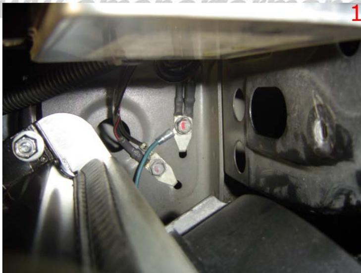
2. Connect the blade connector to one end of the fuse holder and the red wire to the other end using the supplied butt connector. Connect the blade connector to the terminal as shown <sup>2</sup>. Run the wire out of the box to the side of the grommet <sup>3</sup>.
