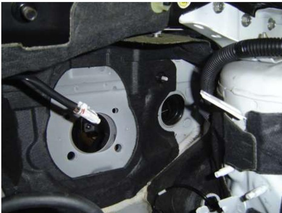
6. Now it's time to pull out some sort of grinding tool that can fit in tight spaces. You will have to grind off the backs of the top-left and bottom-right studs around the clutch master cylinder. These are marked with an X below. Be careful not to grind into the firewall sheet metal. As you get deeper you will begin seeing and outline of the stud. At some point you will be able to push the stud out leaving a clean hole behind.
