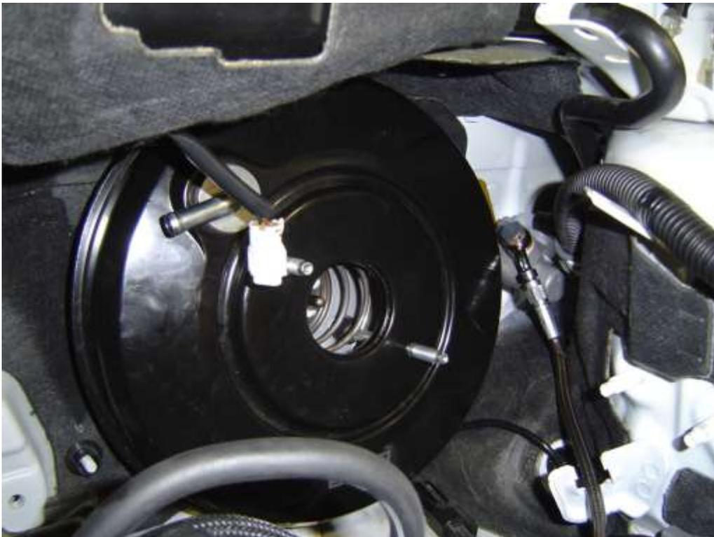
12. Install the brake master cylinder and bleed the clutch and then the brakes.
