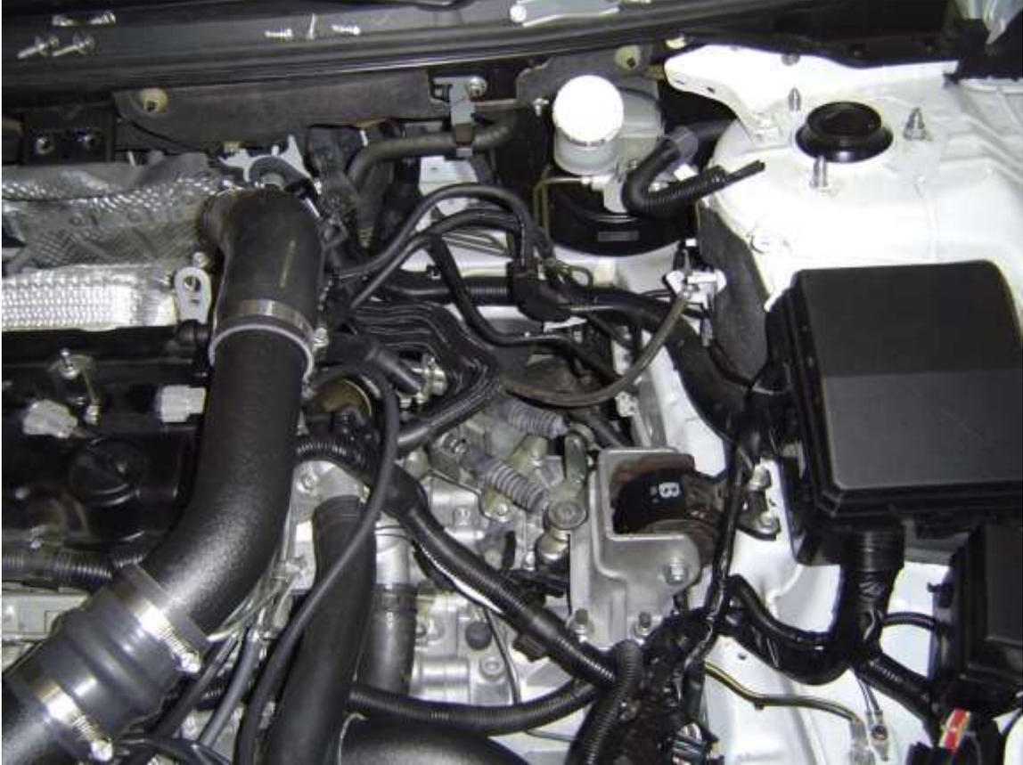
2. Now remove the brake master cylinder. Start by disconnecting the fluid level sensor connector. Then the two hard lines going to it. And finally the two 12mm nuts and pull off the master cylinder. Notice that there is an o-ring between the master cylinder and brake booster. This has to go back on later or you will end up with a large vacuum leak. Make sure to put a lot of shop towels below the master cylinder to soak up the brake fluid and be sure to keep it off of all painted surfaces.
