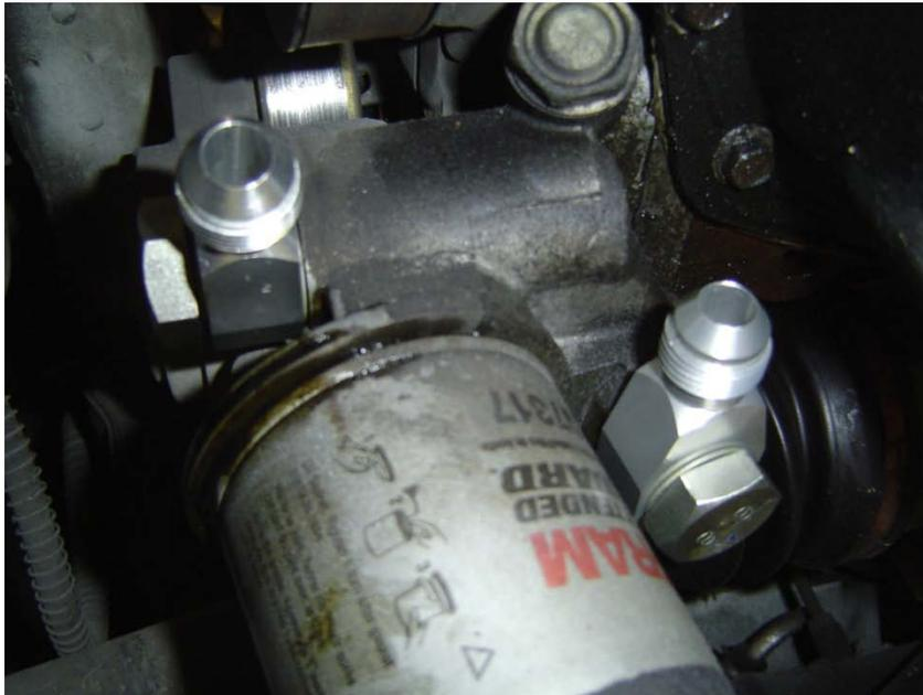
6. You can now install the oil cooler back onto the car and connect the lines to the oil filter housing. The longer line goes to the driver side fitting and the shorter line with the straight fitting goes to the passenger side fitting.
