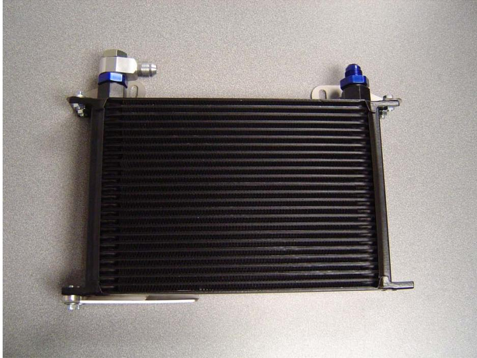
3. At this time remove your OEM oil cooler setup and remove the mounting brackets. Then install them onto the aftermarket cooler as pictured. On the larger bracket that is held on by 2 bolts be sure to install the spacers as pictured.
