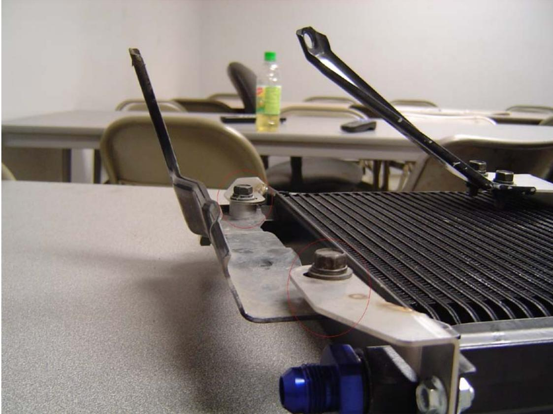
4. You can now install the lines onto the oil cooler as shown, you will want to tighten the top (longer) line before final installation, once installed on the car the line can be very difficult to get to.
