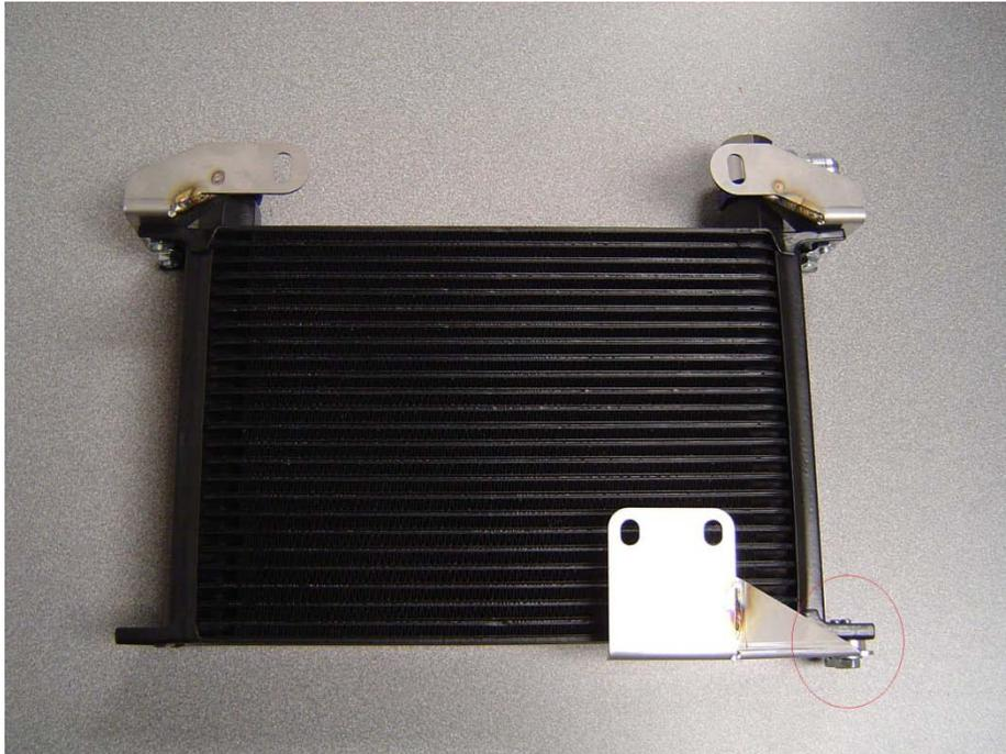
2. Install fittings onto oil cooler as shown, be sure to use the sealing washers on the side that uses the banjo bolt.
