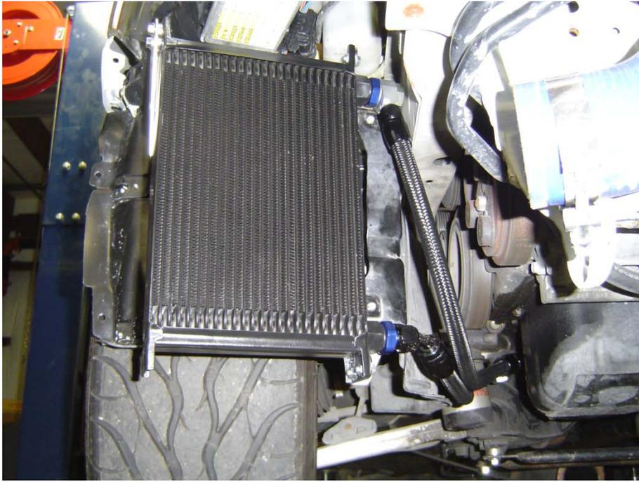
7. Make sure all fittings and connections are tight and check for leaks before driving.
