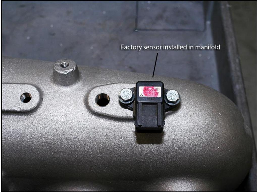
Factory sensor installed in manifold
