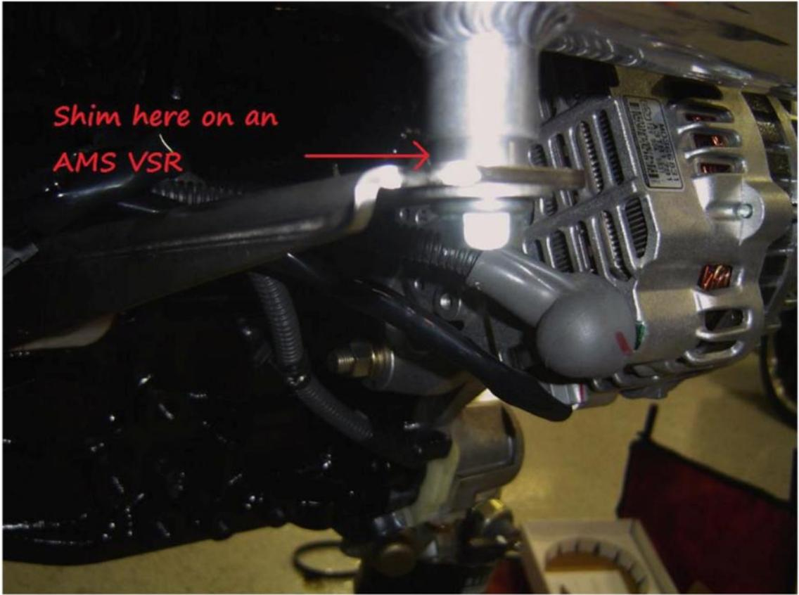
The turbo support bracket will need to be slotted to bolt to the block.
