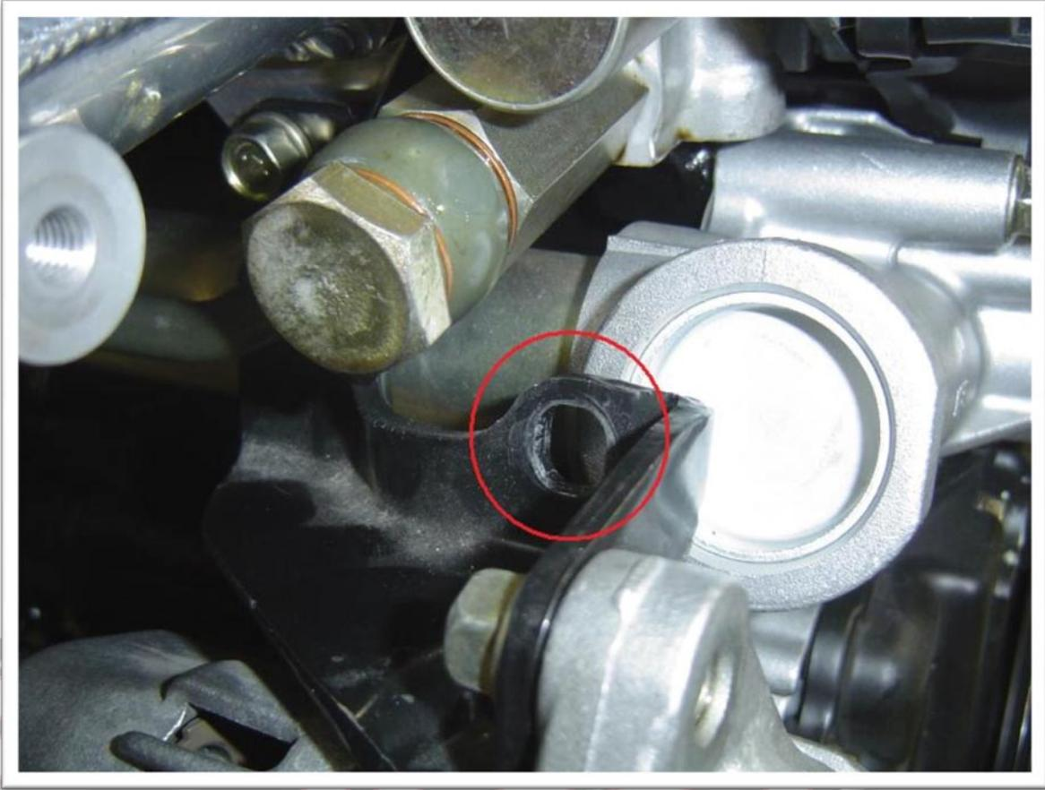
The water pump pulley gets shimmed out slightly with the spacer supplied with the motor.
