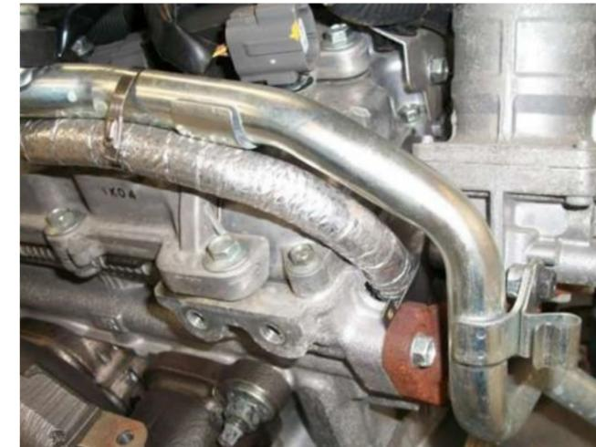
19. Use the supplied metal ties to secure the oil and coolant lines.
