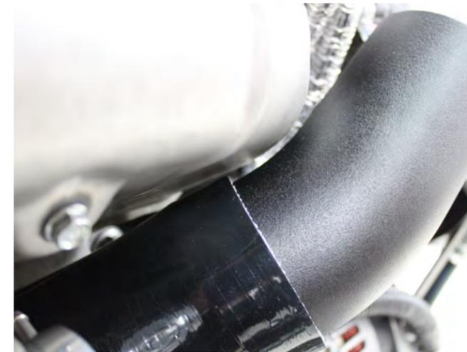
41. Install the turbocharger outlet silicone and metal charge pipe.
