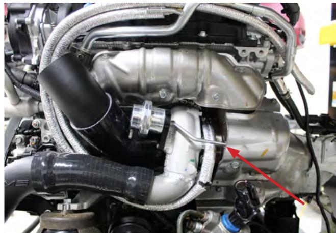
27. Working with the Right/Passenger side now, install the supplied exhaust manifold gasket.
