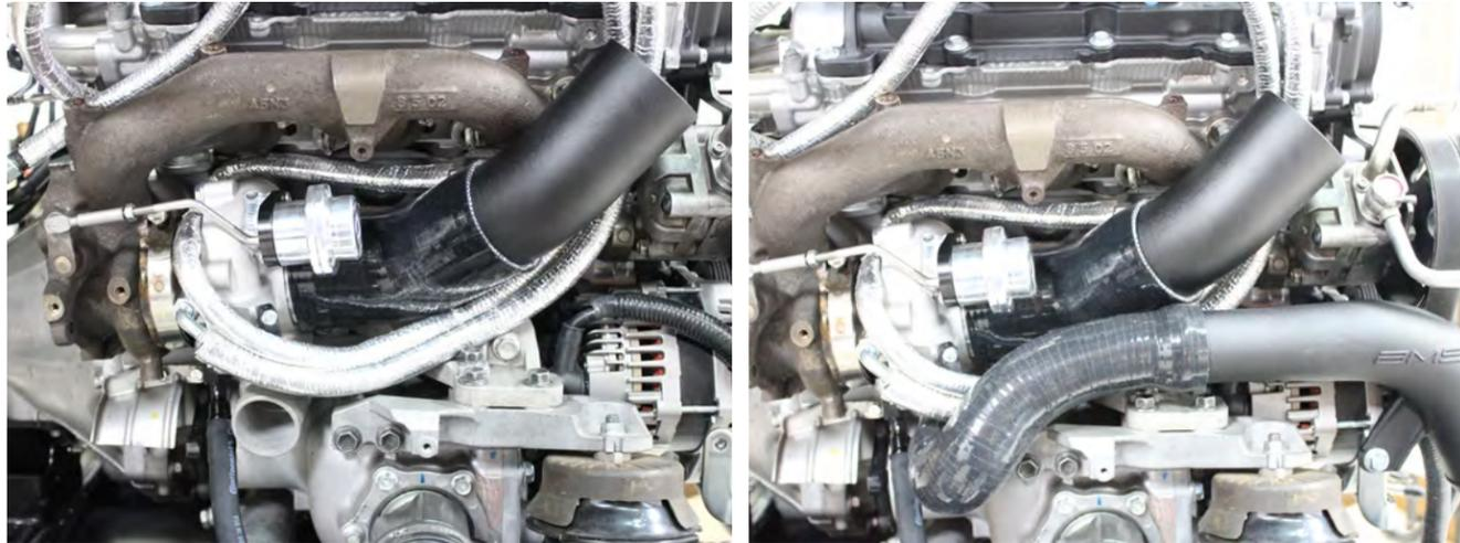
42. Install the remaining heat shields. Check for clearance between the wastegate arms and shields.
