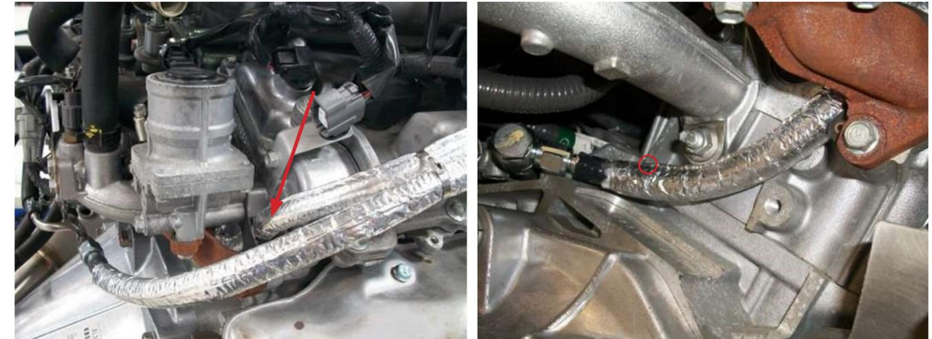
35. Use the supplied metal ties to secure the oil and coolant lines.
