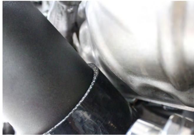
26. Install the remaining heat shields. Check for clearance between the wastegate arms and shields.
