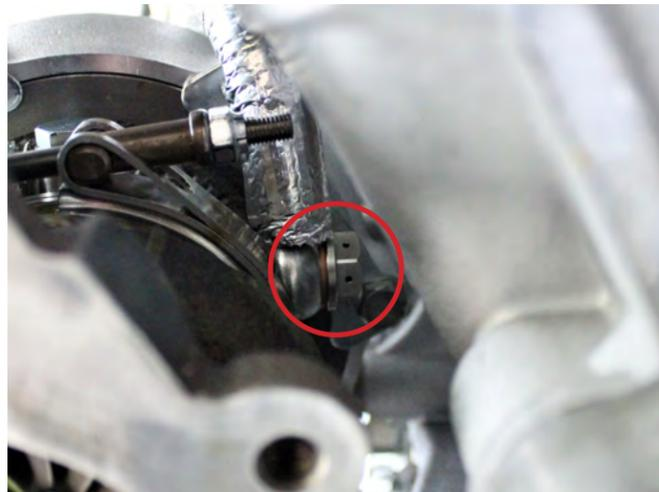
15. Tighten the turbocharger to the cylinder head (reuse factory nuts.)
