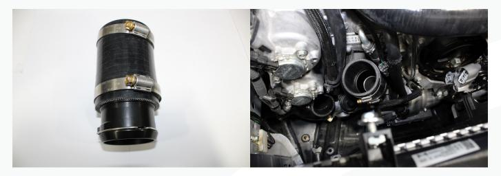
8. Install the lower charge pipe into the silicone on the charge pipe adapter. Leave the clamp loose for now.
