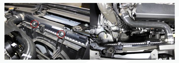
4. Remove the four bolts (circled) and the metal retaining ring(arrow) that hold the TMIC and charge pipe in place.
