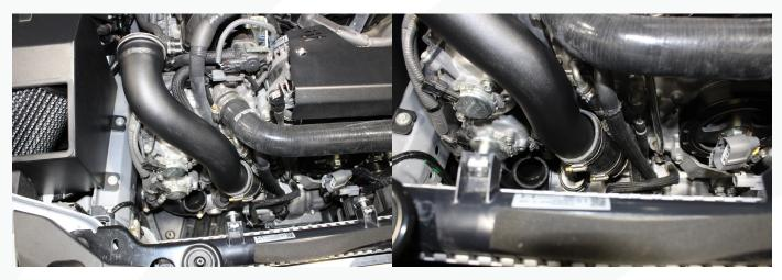
9. Flip the intercooler over and remove the three bolts securing the upper charge pipe.
