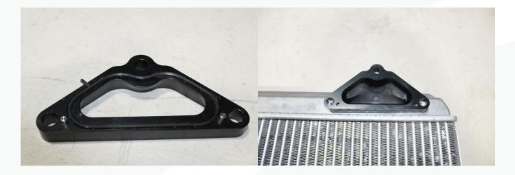
12. Swap the charge pipe gasket from the OEM charge pipe to the new AMS Charge Pipe.
