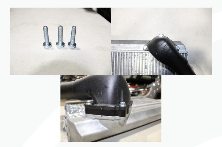
14. Swap the charge pipe gasket from the OEM charge pipe to the new AMS Charge Pipe.
