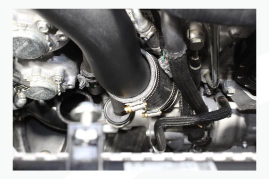
20. Reinstall the cooling fan assembly and any other removed parts. This completes the installation of your AMS WRX Charge Pipe.
