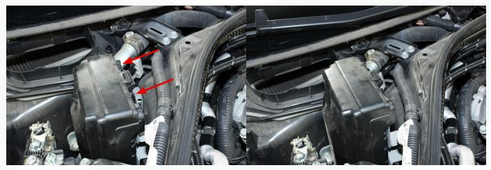
15. Locate the two tabs on the bottom and remove the IPDM cover.
