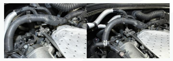
6. Disconnect the fuel line and remove the orange clip and set aside. **They will not be reused.**
