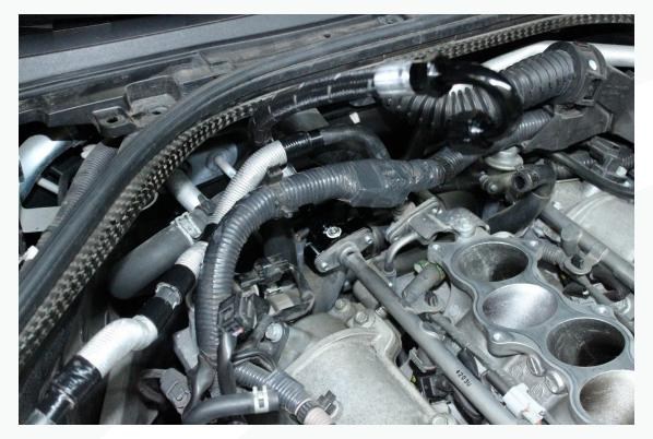
10. Reinstall the intake manifold and torque the bolts to 9ft/lbs. Mount the flex fuel bracket to M6 hole at the back of the intake manifold.
