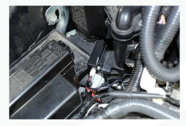
20. Locate the AMS Flex Fuel Harness with the brown 4 pin connector. Plug the brown connector into the flex fuel sensor and route the harness along the fuel line towards strut tower. Secure it with a few zip ties
