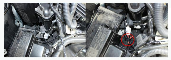
18. Locate the AMS Can Module. It should have 2 connector blanks installed in it already. These are for the optional add-on analog sensors (sold separately). Clean the smooth area of the secondary air injection pump with isopropyl alcohol and adhere the AMS CAN Module to it as shown below.
