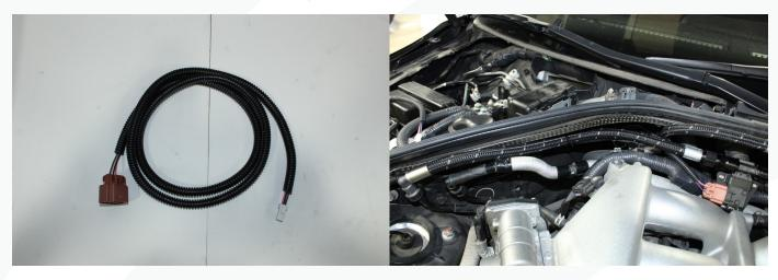
21. Pull the weatherstrip up near the strut tower and spread open the rubber bulkhead and run the harness through with the vehicle harness.
