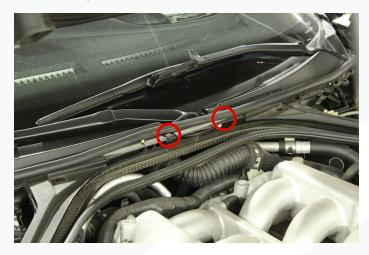
2. On the passenger side, remove the 3 clips holding the upper cowl. Then remove the battery.
