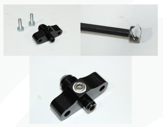
8. Lightly lubricate the o-ring and install the adapter onto the back of the rail. Torque the two M6 bolts to 8ft/lbs.
