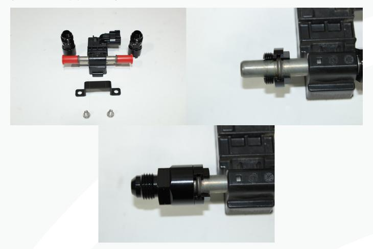
12. Mount the flex fuel sensor with the fittings at the top using the small bracket and M5 bolts to the bracket installed on the intake manifold.
