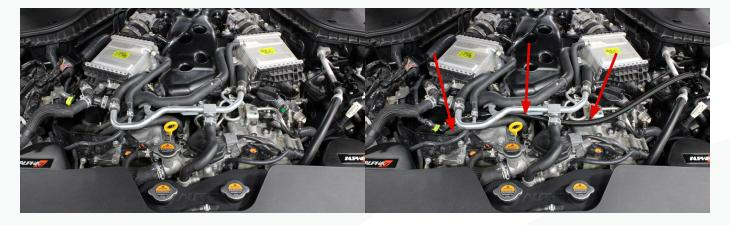
15) Reattach the fuel line to the new bracket as shown on the right side of the engine. Make sure the OEM fuel line is properly clipped into the plastic bracket.
