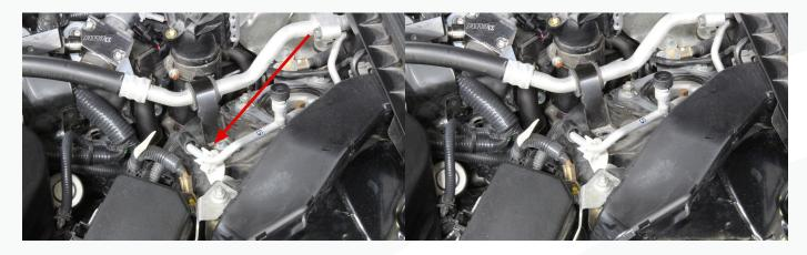
6) Use the supplied M6 x 22mm long button head bolt and install the flex fuel sensor and mount on top of the A/C bracket as shown.
