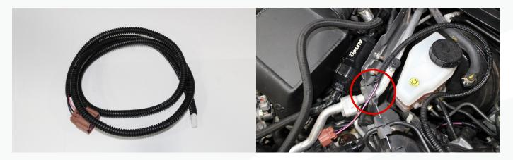
32) Carefully feed the harness over to the CAN module while staying clear of the wiper mechanism and plug it into the CAN module.
