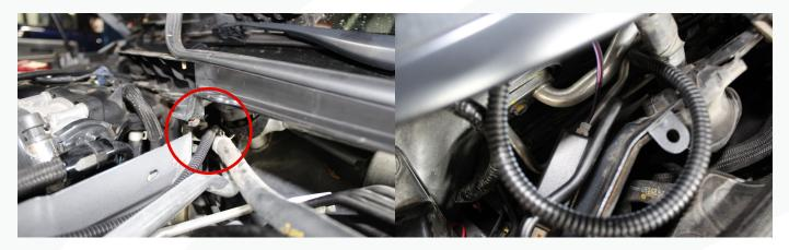
33) Pull slack from the harness to the brake reservoir and secure it to the ac line with a zip tie.
