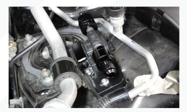
7) Remove the bracket in front of the HPFP. Unclip the harness and fuel line from the bracket. Unbolt the two 12mm bolts from the lower area of the bracket and remove. This bracket will not be reused.
