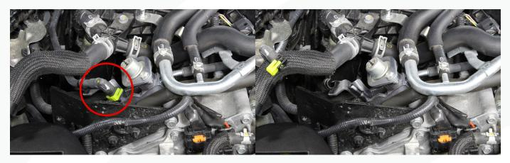
10) Unbolt the fuel line bracket from the engine. It is held in place by two M6 bolts located behind the black bracket shown.
