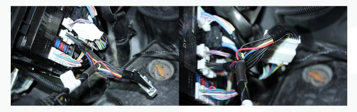
26) Using a zip tie or two, secure the harness neatly so that the IPDM cover can be reinstalled. Route the other end of the harness out the bottom of the IPDM.
