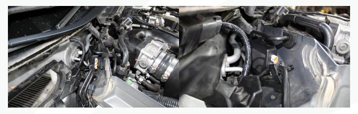
30) Locate the short jumper harness and plug the white 4 pin connector into the box. Then plug in the black 4 pin connector into the main harness.
