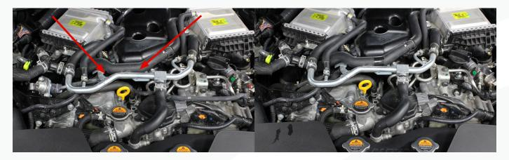
12) Locate the new low-pressure fuel line bracket. Swap the plastic fuel line clip from the OEM fuel line to the new bracket in the same orientation.
