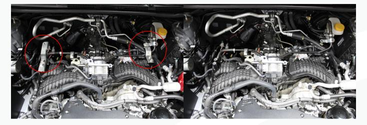
9. Remove the clip holding the washer fluid filler neck to the body. Be sure the washer fluid level is below the filler neck, so it does not spill and remove it.
