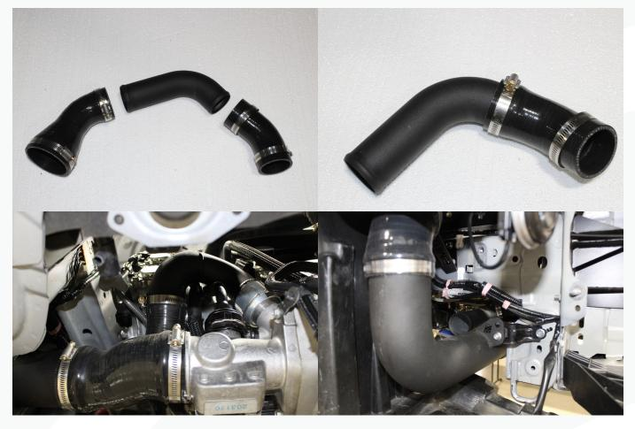
33. Install the adapter silicone to the end of the pipe and position it as shown below.
