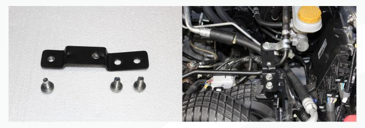
40. Locate the throttle body adapter and the provided M8 hardware. Install the o-ring from the TMIC into the throttle body adapter and install the adapter onto the throttle body. The shorter M8 bolt should be used on the threaded adapter hole (circled below).
