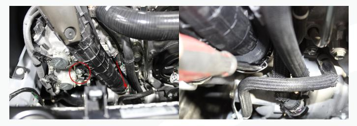
6. Remove the charge pipe retaining ring and o-ring from the oem charge pipe and set it aside as it will be reused in a later step.
