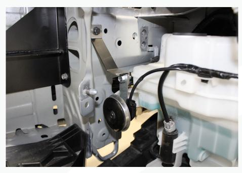
26. Mount the provided Ambient Temp Sensor mounting bracket to the vehicle stud. Remove the harness clips and reroute the harness along the radiator support and clip the sensor into the front of the bracket.
