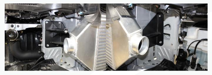
30. Install the metal retaining clip and o ring from step 6 onto the C shaped charge pipe.
