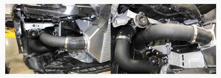
37. Connect the drivers side charge pipe and silicone. Reuse the crash beam nut to mount the charge pipe to the stud.
