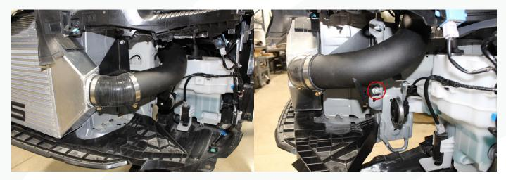
38. Install the straight hump silicone with (2) #48 clamps onto the charge pipe near the battery. Line up the groove on the inside of the silicone with the tube and tighten the lower clamp.
