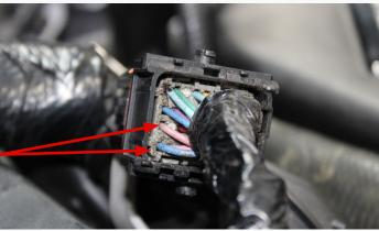
33) Carefully cut back some of the tape/loom to gain access to the wires in order to splice into them.
