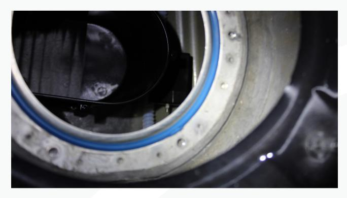
56. Connect the short hose created in step 39 to the siphon block on the fuel pump assembly.
