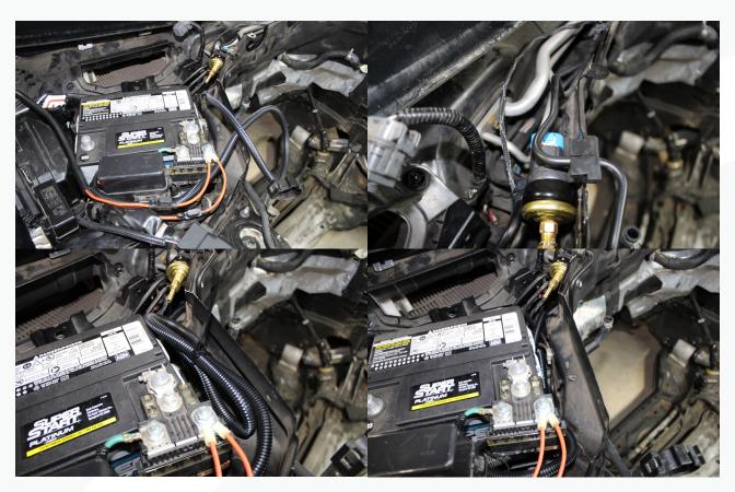
99. Locate the 5mm hose, clamps, and barb fittings. Install one clamp to the hose and then secure it to the hobb switch.
