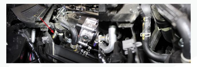
104. Place one more clamp on the small section of hose, then push the open barb onto the hose that was just removed and clamp it. Then install the new hose on the intake manifold barb and tighten the clamp.
