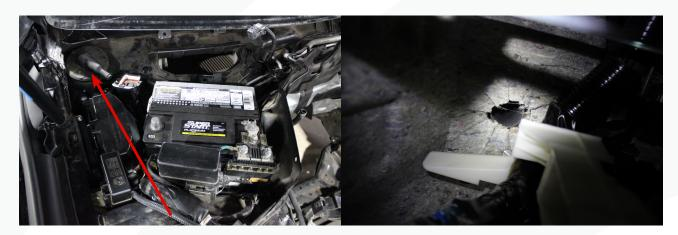
85. Trim the grommet just before it enlarges. This spot will fit tight on the loom to help prevent leaks.
