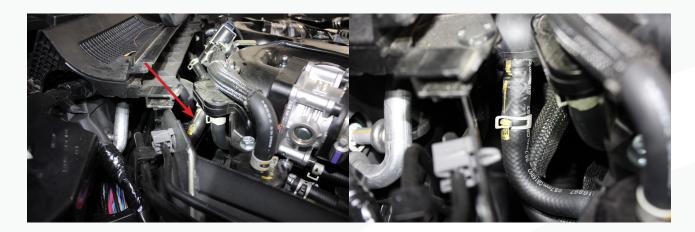
93. Place one more clamp on the small section of hose, then push the open barb onto the hose that was just removed and clamp it. Then install the new hose on the intake manifold barb and tighten the clamp.
