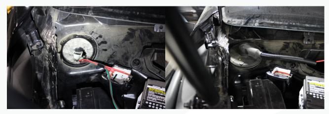
87. If necessary, pull back some slack of the loomed harness and secure it to a nearby harness in the passenger kick panel.
