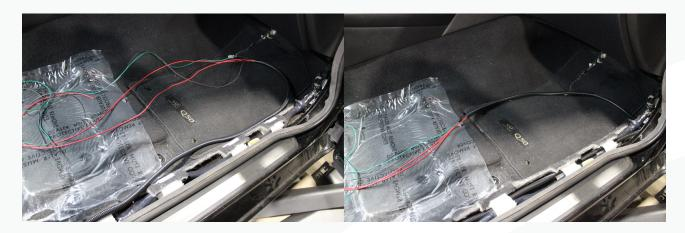
84. Locate the vehicle grommet near the battery. On the underside of the dash, release the plastic tabs under the insulation holding it in place.
