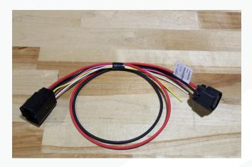
63. Cut back some of the wire loom on the factory top hat connector.
