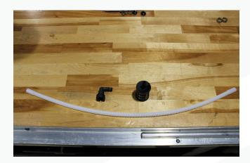
41. Assemble the hose as shown below, using the cinch clamp on the siphon strainer. Again, using a small amount of heat without damaging the hose, affix the 3/8 quick connect fitting to the other end of the siphon hose. Measure 6" from the strainer, fix the magnet to the hose with 1 zip tie.
