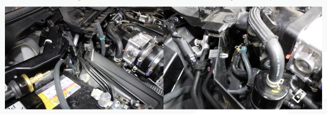
96. Route the hose with enough slack for engine movement back to the hobbs switch on the battery. Trim the hose and secure it with a clamp. **Then skip to step 106.**
