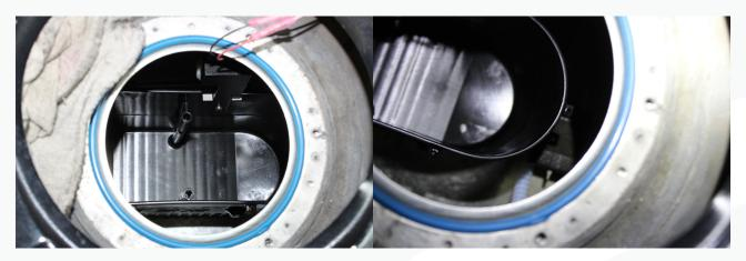
54. Set the basket near the opening in the fuel tank and connect the level sensor.
