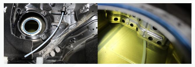
45. Install a 11.3 Oetiker clamp onto the end of the hose and push the open end of the hose onto the metal tube at the front of the tank. Cinch the clamp with Oetiker pliers to secure the line to the tube.
