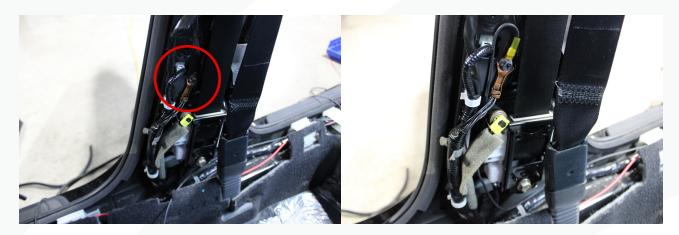
80. Locate the two-wire hobb switch extension harness and plug it into the open connector on the relay harness.
