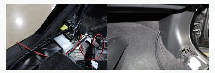
82. Starting at the b pillar, slide the split loom over the red and black wires towards the relay.
