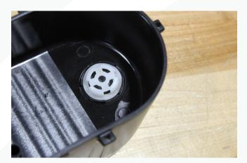
37. On the side of the basket there will be two dimple features. The Q50/60 you will need to drill the top hole with a 13/64 drill bit. On the Z the basket has three tiers, so you will need to drill both the holes on **only** the top tier.
