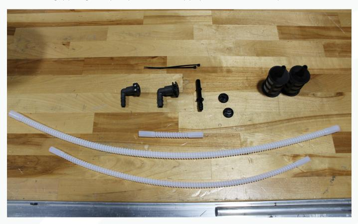
39. Assemble the small siphon adapter hose using the 5/16 90 degree quick connect fitting, siphon hose and adapter fitting. Carefully apply a little heat to the end of the hose using a heat gun to fully seat the siphon hose. Too much heat may permanently damage the hose. Install the green quick connect clip on the siphon adapter.
